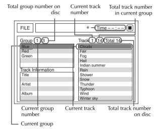
\* Elapsed playing time of current track Elapsed playing time is only shown during playback.
